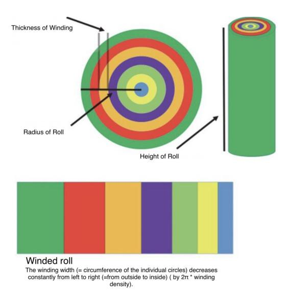
Figs. 46-47: Closed roll in longitudinal and cross-sections, and wound roll.
